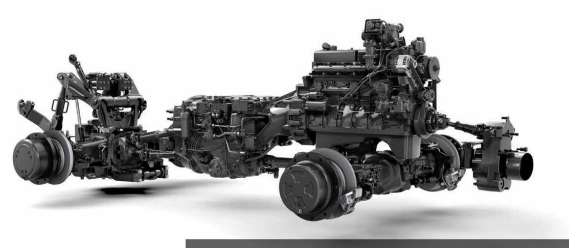
CVT transmission ensures optimum use of power and torque, with seamless acceleration and power delivery, ideal speeds for every situation, and ultra-fine speed control for top-quality work with all implements.
